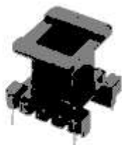
Ho Sung International. EI-2820 nylon bobbin. Core is 10 mm x 13 mm x 10 mm high. Top is 18.5 mm x 21.5 mm. Base is 22 mm x 26 mm. Four leads, 15 mm and 20 mm spacing
