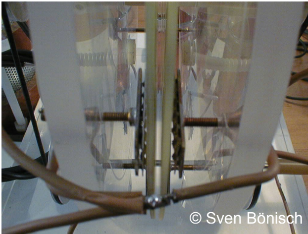
Fig. 5: Electrode setup at the terminals HV1 and HV2
